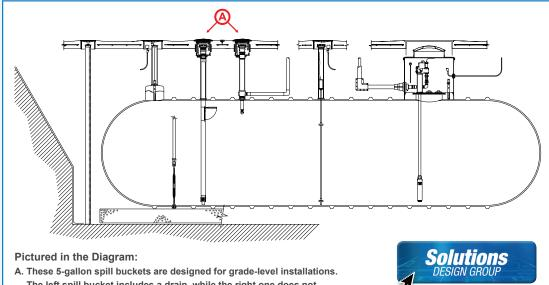
The left spill bucket includes a drain, while the right one does not.
